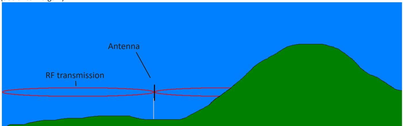
This diagram visualises the RF transmission pattern being absorbed by mountainous terrain.
