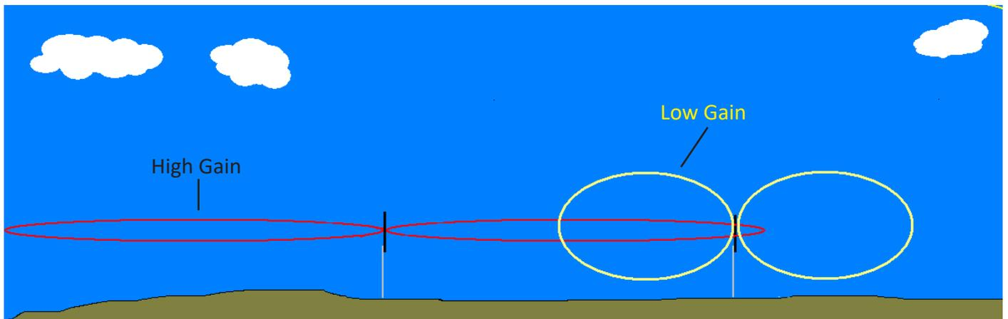
This diagram visualises the use of a Low-gain antenna, note that the beam width is significantly shorter and unable to reach the RF destination in addition RF energy is being wasted radiating into a wide beamwidth.
