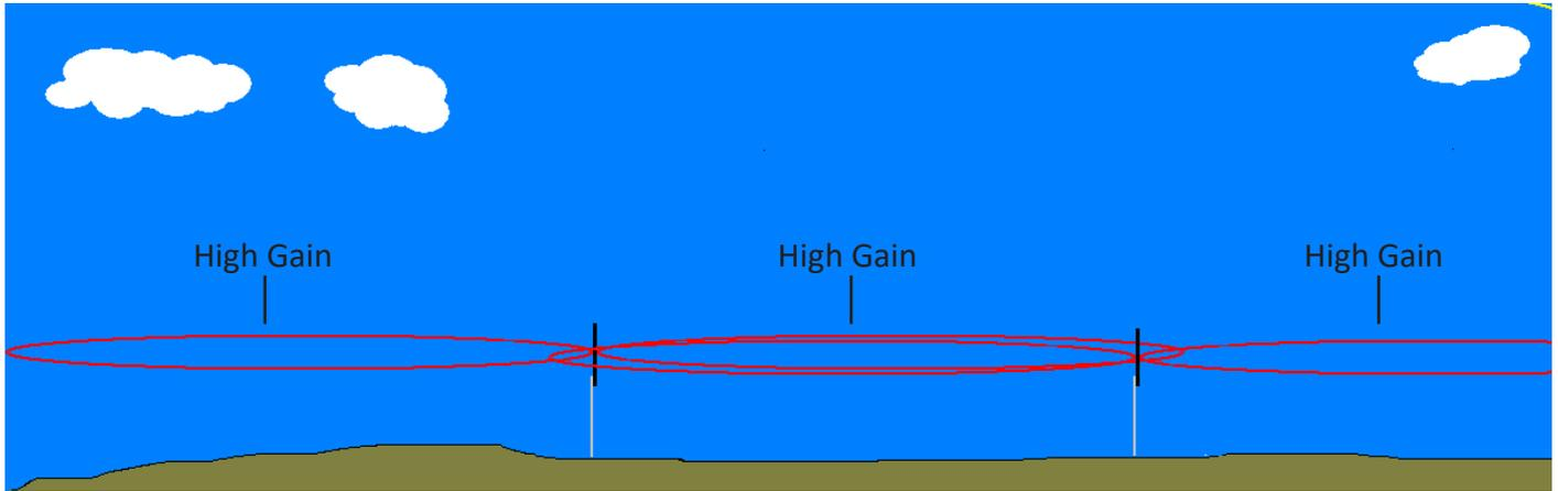
The above diagram visualises the use of high gain antennas utilised in a flat location **NOTE:** long thin beam width enabling RF communications between sites.
