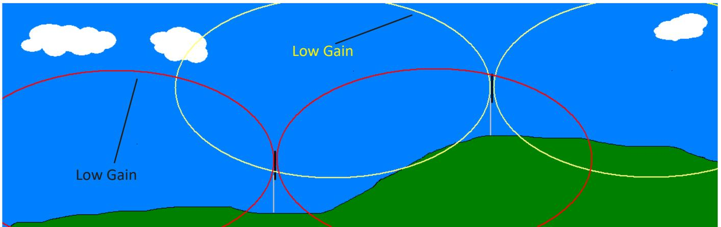
The above diagram demonstrates the correct antenna selection, here a low gain antenna is utilised at the telemetry site. **NOTE:** the wider beam width allows RF radiation to be directed in an upward direction and is able to reach to hill top above.
