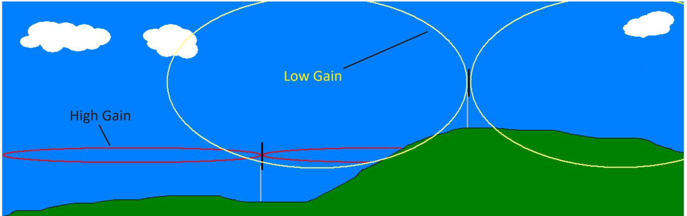
The above diagram demonstrates the effect of using a hi-gain antenna in a valley, **NOTE:** the beam width is narrow, and unable to reach the hilltop above.
