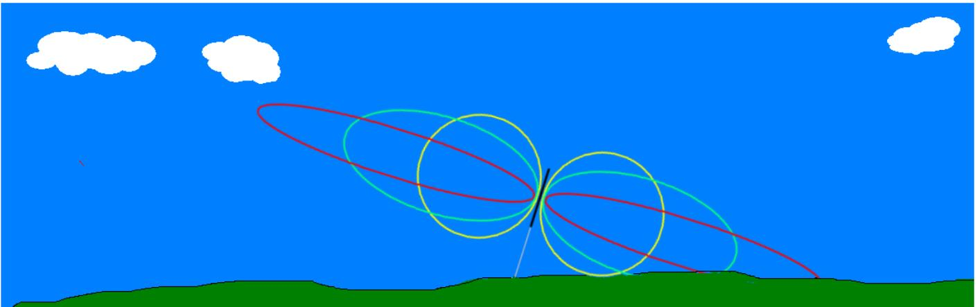
This diagram visualises the effect of an antenna that is not mounted in a vertical position. **NOTE:** that the RF transmission is radiated toward the Earth and Sky
