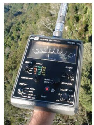
RF field test meter with sensitive RF cone attachment
