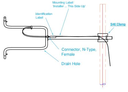
**FMD-CPLP-L Array 3-Stack Array** with **Power Divider**
