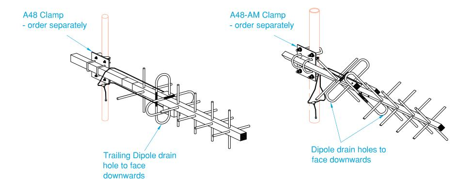
**Mounting of Yagi Antenna** - Horizontally / Vertically Polarised **Mounting of Yagi Antenna** - Cross Polarised
