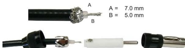
4. Place the retention clip over the end of the cable and exposed braid, then squeeze the fingers into the cable jacket to hold the clip secure.
