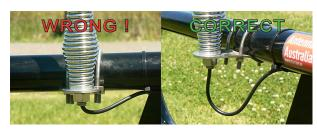
Important installation tip: Check the condition of your coaxial cable. Ensure a stress relief loop in the cable leaving the spring base. This will permit the antenna to flex in the usual manner during travel, without placing unnecessary tension on the cable.
