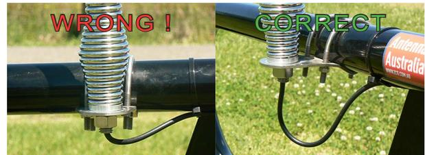
**Failure to follow this advice will most likely result in the feeder cable being ripped out of the antenna ! The issue is not covered under warranty.**
