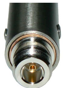
N-type female termination at base of mount section
