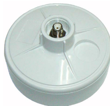
TNC female bulkhead termination in base of dome antenna. Will require additional water sealing via amalgamation tape and PVC tape
