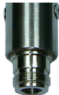
N-type female in base of mount section
