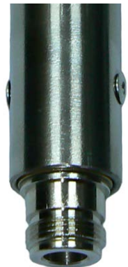
N-type female in base of mount section
