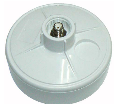
TNC female bulkhead termination in base of dome antenna. Will require additional water sealing via amalgamation tape and PVC tape
