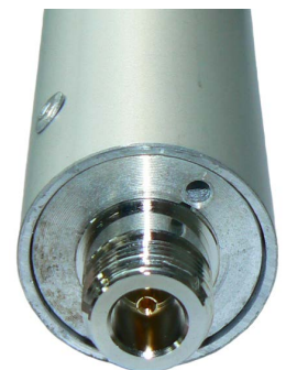
N-type female in base of mount section
