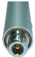
N-type female in base of anodised aluminium mount section
