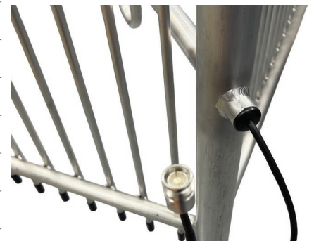
RA4-R 4.3-10 female connector in rear of dipole
