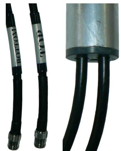
Dual cable and terminations
