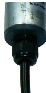
RG213 exit from base through cable sealing gland.
