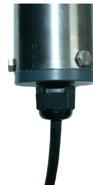
Coaxial cable exit from base through sealed cable gland
