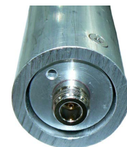
N-type female in base of ruggedised aluminium mount section
