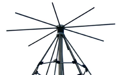
Upgraded radials and head with radial supports
