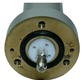
7/8" EIA input at base of power divider
