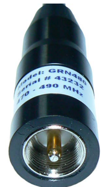
UHF male embedded into mount ferrule
