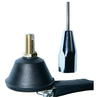
Detachable whip. OB base must be installed prior to fixing whip onto base. Must have metallic ground plane to work at stated levels.
