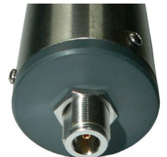
N-type female fitted to rear of antenna
