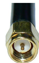
SMA male termination as base of whip
