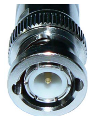
BNC male termination as base of whip
