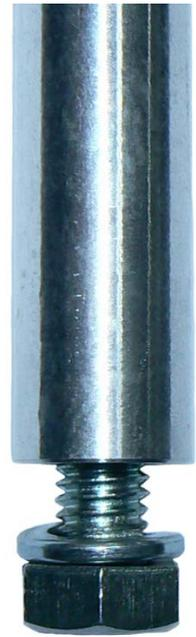
Alternatively: For A-4266-4 adaptors only, you can mount using the spring base bolt in the bottom 1/2"-12BSW thread into a 12.7mm hole or suitable bracket. If antenna didn't have spring base such as SGDB-TPM please purchase a A-4266-4-B which includes a 1/2"-12BSW bolt with spring washer.
