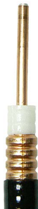
Suits 1/2" flexible, corrugated copper shielded, foam PE dielectric, solid conductor cable - ZCG1250
